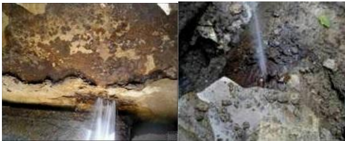
Figure 4. DH pipeline accidents in case of external corrosion [11]
