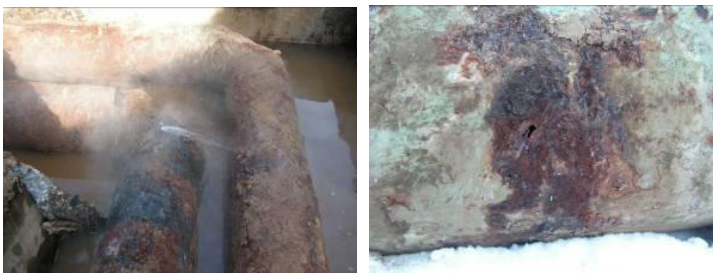
Figure 5. Kaunas DH pipeline accidents in case of external corrosion
